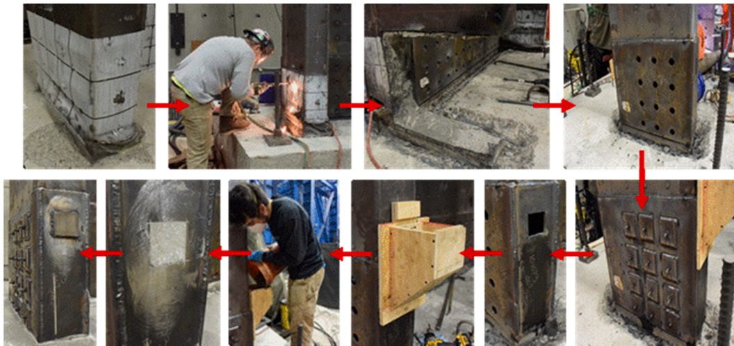
Fig. 8. Repairing sequence of webs.
